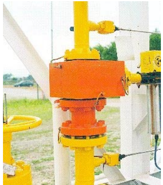
A typical I-SEP unit, capable of handling 6,000 barrels of oil per day
