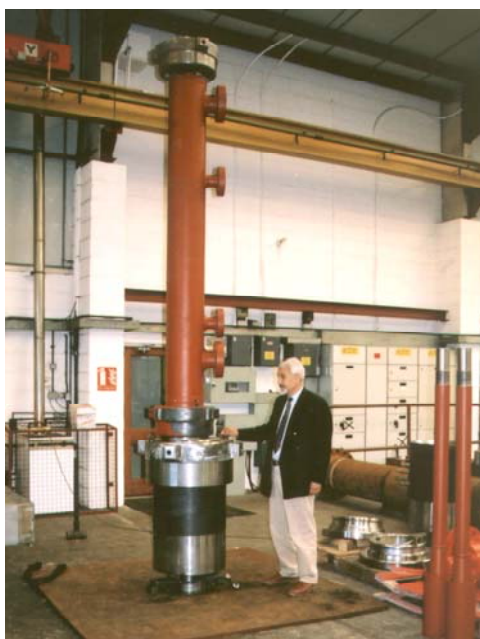
FIG 11. CALTEC'S COMPACT SEPARATOR I-SEP WITH INTEGRAL LIQUID KNOCK-OUT VESSEL (I-SEP)
